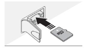
Figure 2.10 Installing the MicroSD Card
