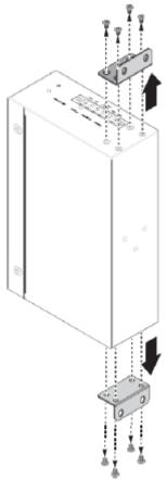
Figure 2.4 Installing Wall Mount Plates
