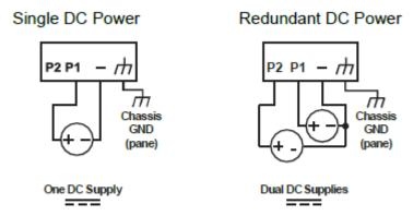
Figure 2.12 Power Wiring for JetLink Seies
