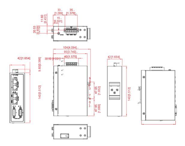
Figure 1.7 Dimensions (JetLink1102/1302)
