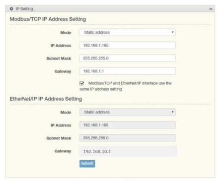
Figure 3.11 Network Setting > IP Setting
