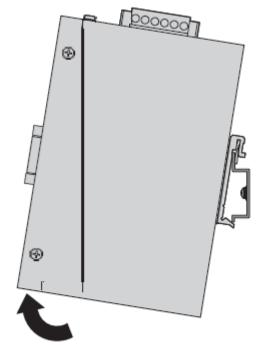
Figure 2.3 Removing the DIN-Rail
