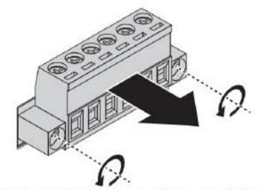
Figure 2.16 Removing a Terminal Block
