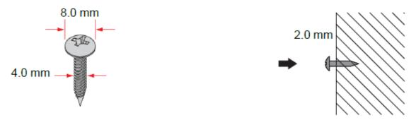
Figure 2.5 Securing Wall Mounting Screws
