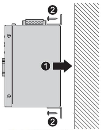
Figure 2.6 Wall Mount Installation
