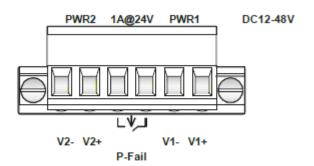
Figure 2.15 Terminal Receptor: Power Input Contacts
