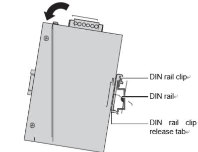
Figure 2.1 Installing the DIN-Rail Mounting Kit-
