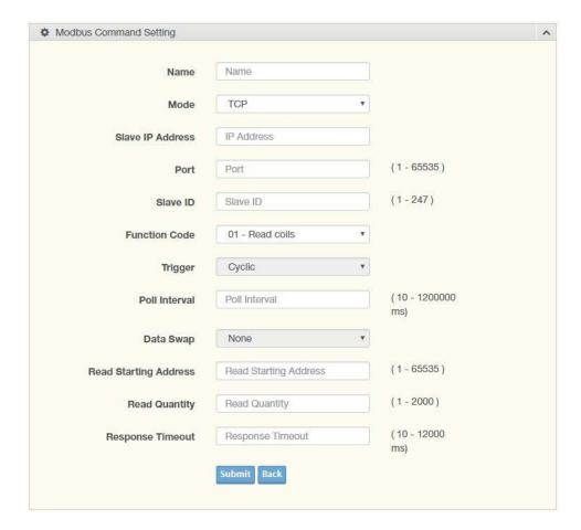
Figure 3.18 Protocol Setting > Modbus Setting > Add
