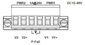
Figure 2.14 Terminal Receptor: Relay Contact
