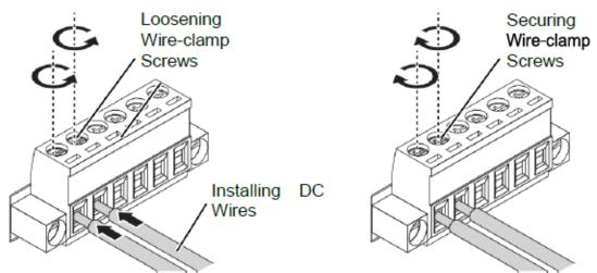
Figure 2.17 Installing DC Wires in a Terminal Block
