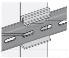
Figure 2.2 Correctly Installed DIN Rail Kit-
