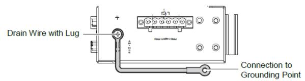
Figure 2.13 Grounding Connection
