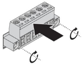
Figure 2.18 Securing a Terminal Block to a Receptor
