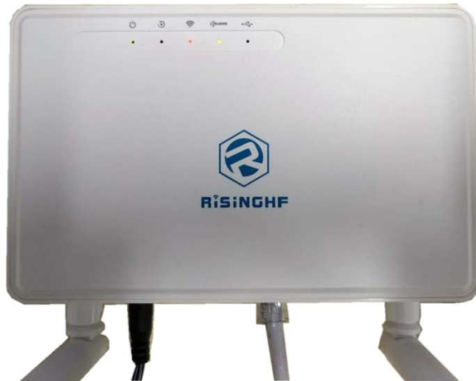
Figure 3-5 Led instructions in default AP mode when connected to cloud server
